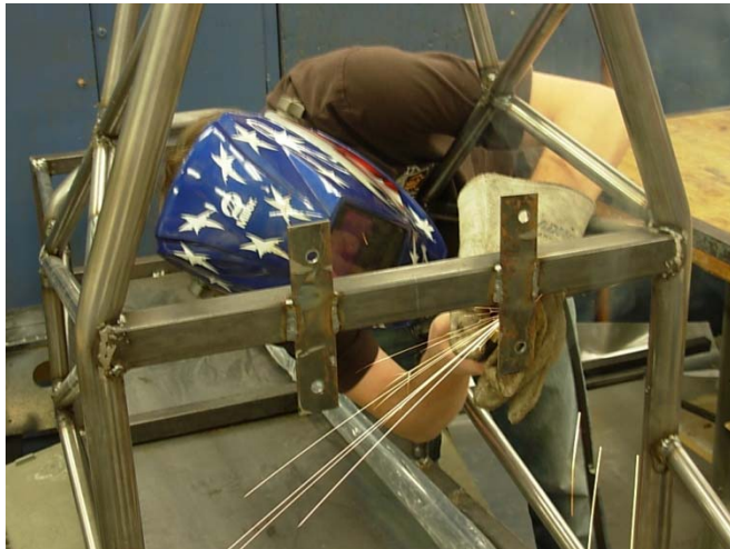
Connor welding the mounts for the fuel tank
